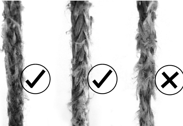
Figure 2-4. Examples of new, acceptable and unacceptable ropes
