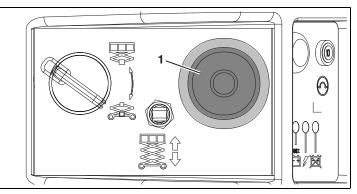
Figure 4-4. Ground Control - Emergency Stop Switch
