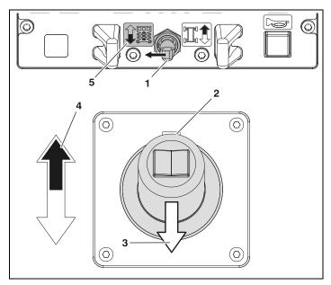
Figure 4-7. Raising Platform From Platform Control
