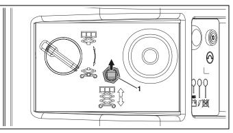
Figure 4-6. Raising Platform From Ground Control
