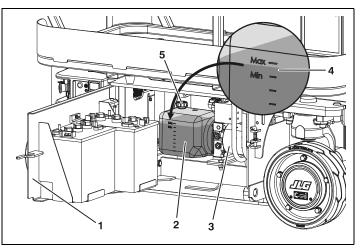
Figure 6-1. Hydraulic Oil Check Procedure
