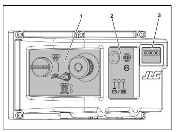
Figure 3-2. Ground Control Station
