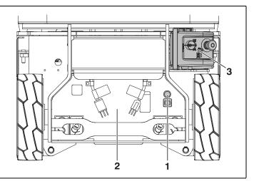
Figure 3-6. Location of Brake Release Switch (Rear of Machine)
