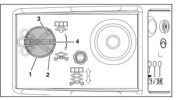
Figure 4-3. Platform/Ground Select Switch
