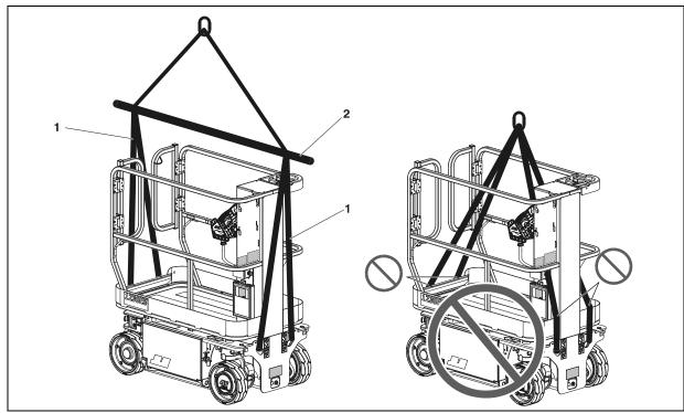
Figure 4-15. Lifting Using Spreader Bar.
