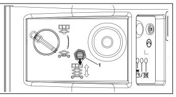
Figure 4-8. Lowering Platform From Ground Control
