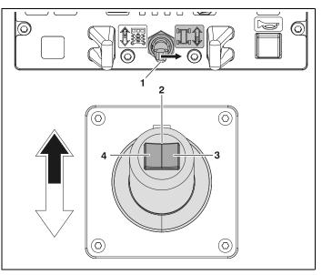
Figure 4-10. Steering from Platform Control
