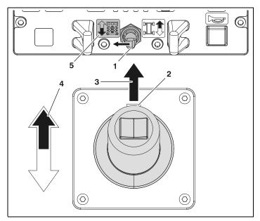
Figure 4-9. Lowering Platform From Platform Control
