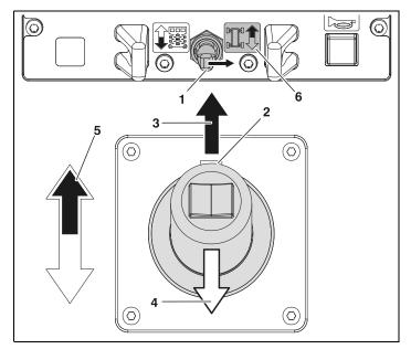
Figure 4-11. Driving Forward from Platform Control
