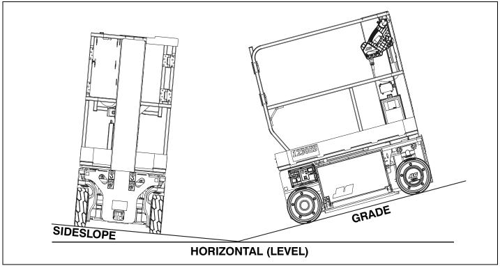
Figure 4-12. Grade and Slideslope Definition
