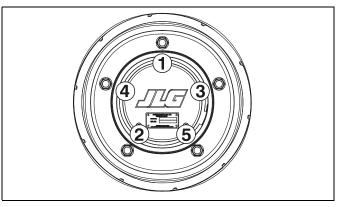
Figure 6-3. Wheel Lug Nut Tightening Sequence
