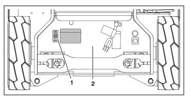
Figure 4-2. Location of AC Inverter ON/OFF - Toggle Switch
