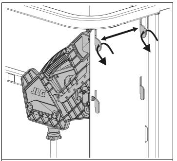
To prevent unauthorized removal, the platform control station can be secured to it's mount by placing a lock through one or more of the holes located on it's upper mounting tabs.
