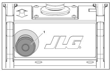
Figure 4-5. Platform Control - Emergency Stop Switch
